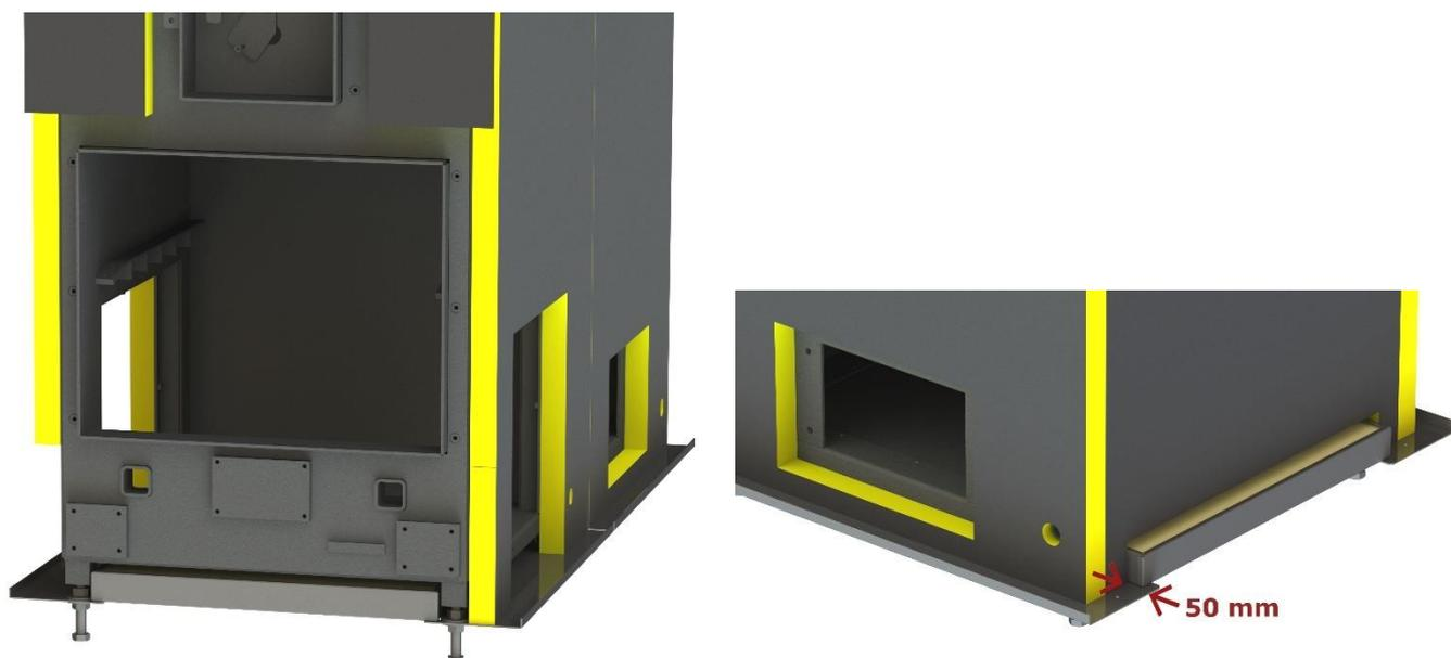
8. Insert and screw fuel feeder into the combustion chamber. The side of the inlet fans is screwed directly into the combustion chamber; an auxiliary flange must be used on side of outlet of ash worms.
