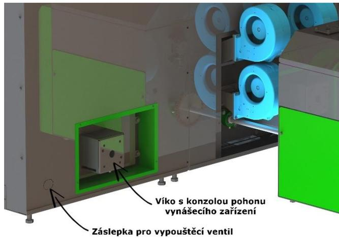
26. Insert the worm with electric gearbox and screw them to the bracket. The worm shaft is secured against sliding by an M10x25 screw and washer 10. If automatic deashing is not used, the opening is closed by an inspection lid
