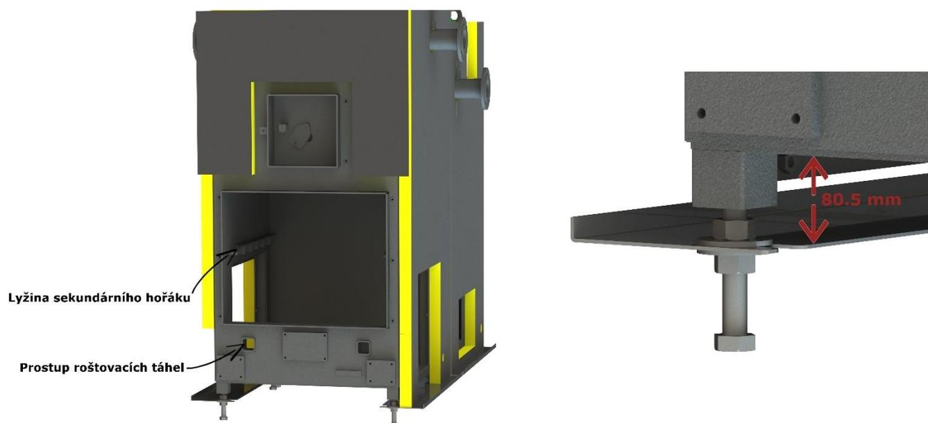
7. Insert insulated sheets under the boiler. Leave 50mm space on the rear side of the exchanger for the rear part of the outer casing.
