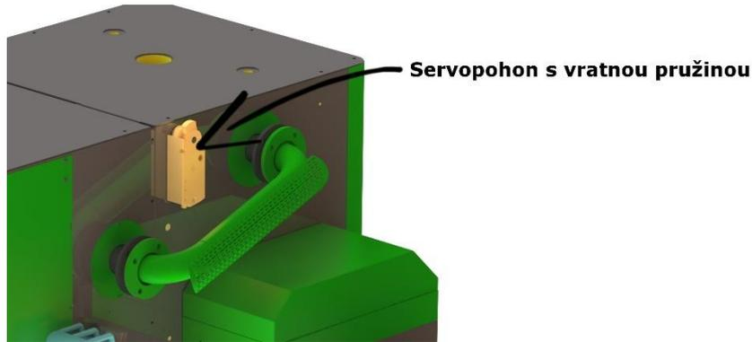
33. Install and screw the separation fire flap together with actuator fitted with a return spring on the fuel bin. Screw the flap to the top of the intermediate bin after the channel of discharge equipment is seated. Assembly of the actuator with the flap axis must ensure that the flap securely closes when the actuator is without control voltage.
