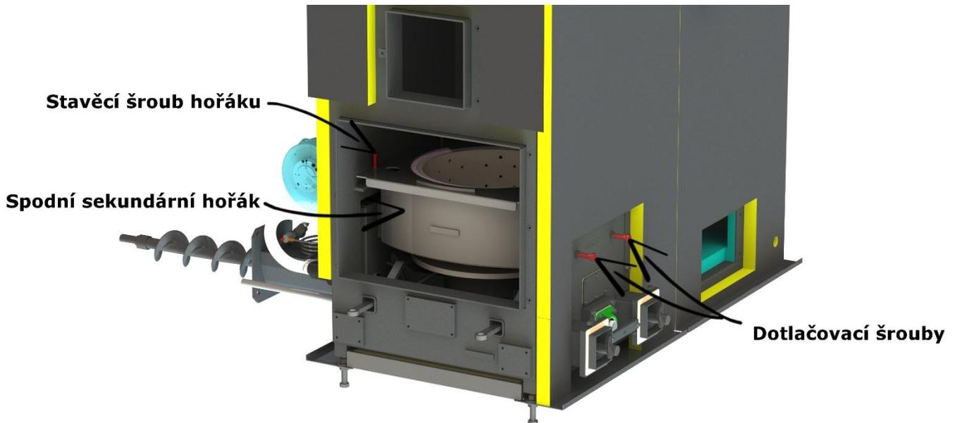
12. Put a refractory deflector on the secondary burner in the combustion chamber. Handle the ceramic deflector very carefully.
