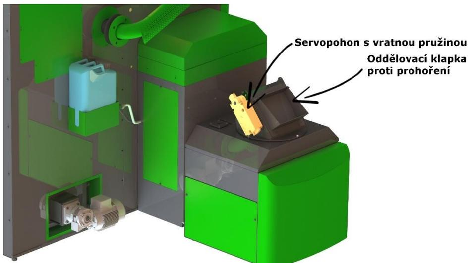
34. Set up the fuel conveyor according to the drawings for the deployment of the technology and lock it together with the separation fire flap. Fill the opening between channel end and the separator flap with silicone.
