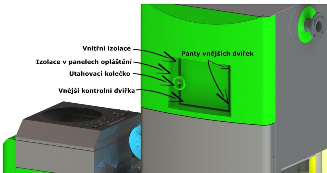
22. Install heat exchanger and put casing on it. Insulation must be installed to sheet metal panels. Rear part must be aligned with the support rails.
