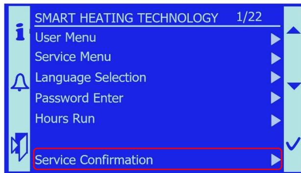
When this message appears, operator of the equipment is obliged to perform the prescribed inspection tasks and the maintenance of the equipment. Service is confirmed by the
