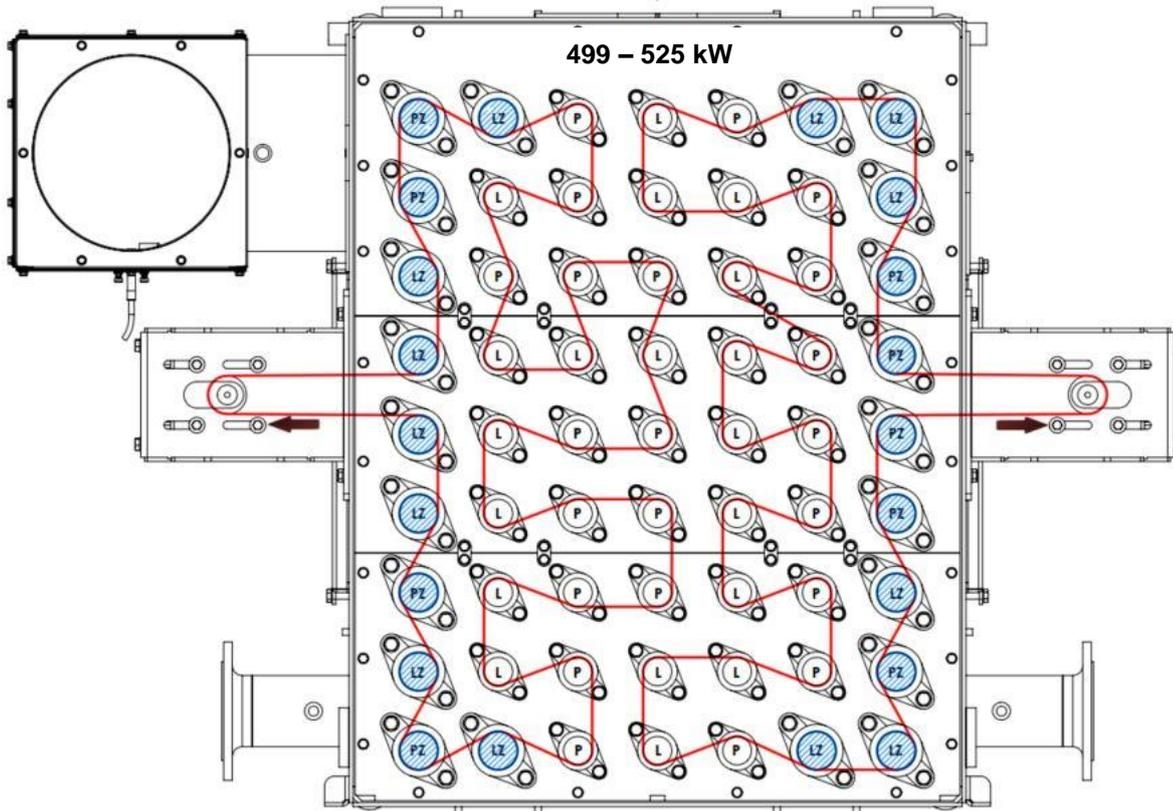
Note: The blue colour indicates the turbulators with reinforced shaft
