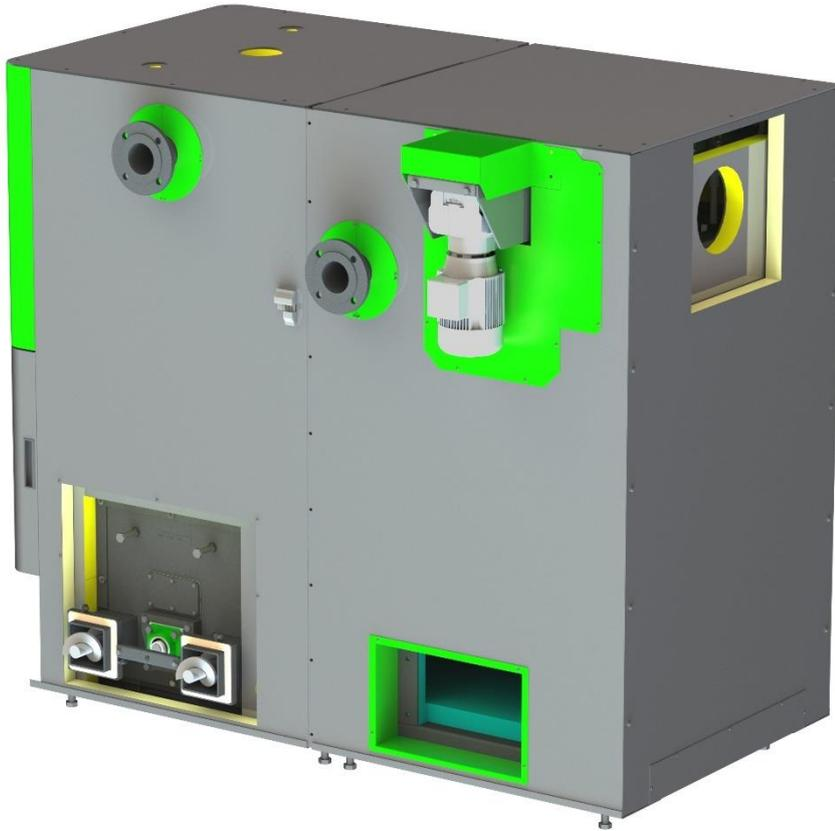
23. Screw the chimney body on. The chimney body is fitted with a well for the sensor of exhaust gas temperature and lambda probe. A Teflon seal must be glued between the heat exchanger and the chimney body. The chimney body can be fitted from the rear, left or right. For this variability of installation, the manufacturer has prepared mounting holes and cover sheets for boiler casing.
