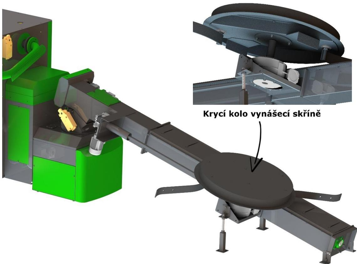
37. Screw the leaf springs assembly onto the main fixed arms of the discharge device. Never shorten leaf springs according to the size of the external fuel store. All bolts shall be loose and shall allow for the sliding movement of the individual spring leaves. This does not apply to the screws securing the leaves to the fixed arms of the discharge wheel.
