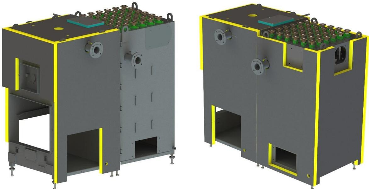
6. Nuts and fender washers are prepared on the adjusting legs, between which the skids are attached that bear the outer casing. Both skids must be at the same height and level with the boiler. The internal dimension between the boiler bottom and the skid is 80.5mm
