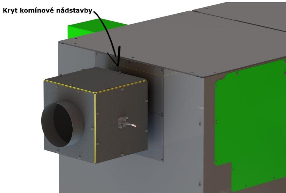
25. Screw the lid to the heat exchanger, which bears a bracket for drive of the deashing device (or the inspection lid of exchanger).
