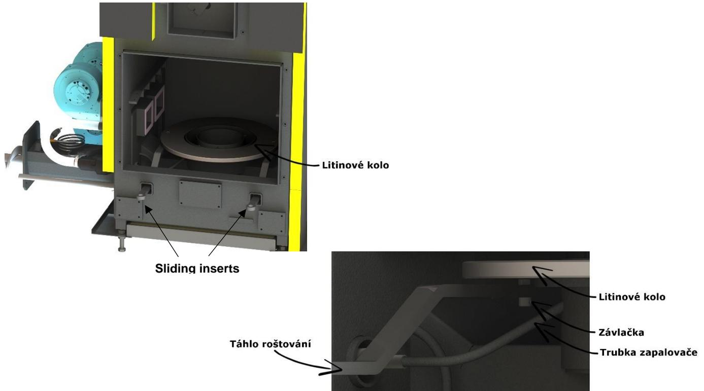
10. Insert cast iron primary burner inserted into the annular ring of the feeder and secure it with three spring pins. The primary burner must not prevent the cast iron grate wheel from moving.
