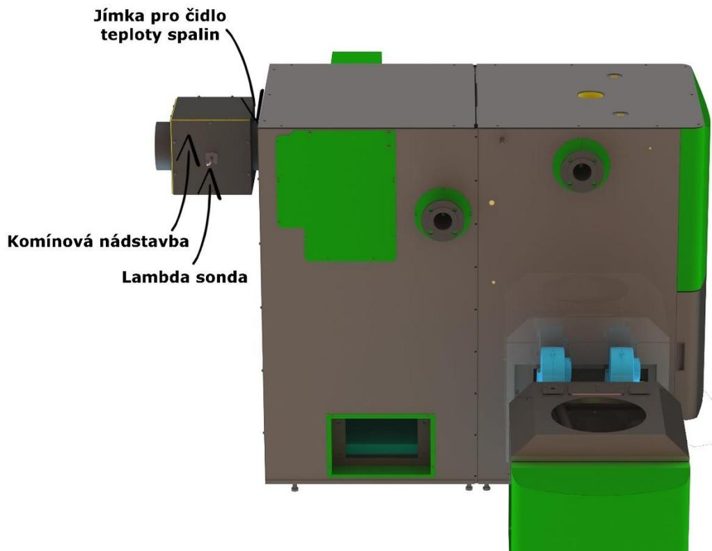
24. Screw on the cover plates around the chimney body
