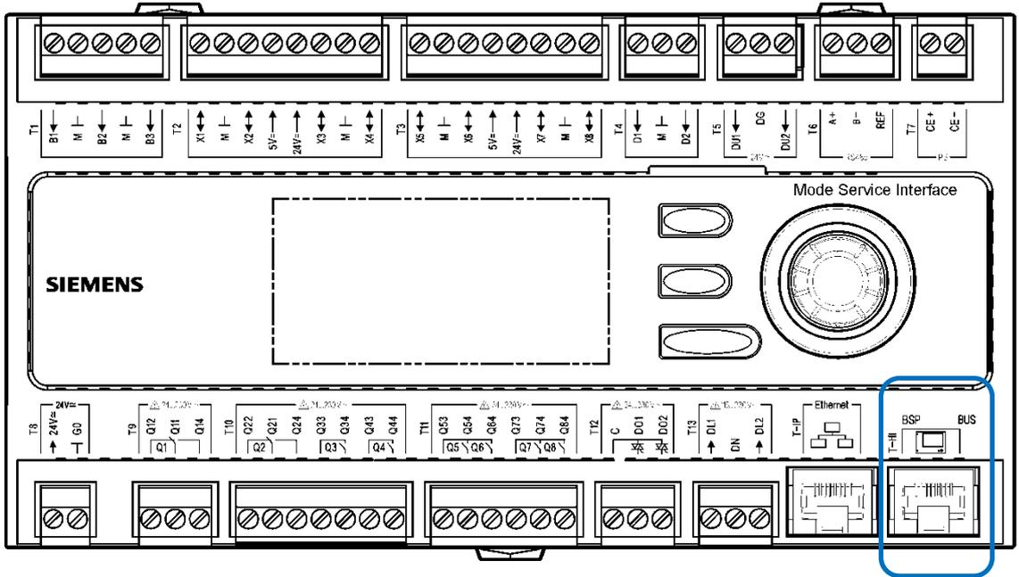
2. The controller has a factory default IP address of **192.168.1.42**
