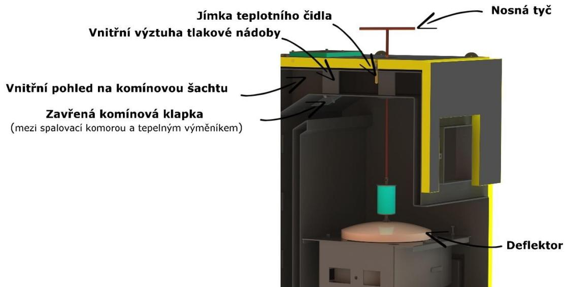
14. After securing the deflector, pull it to the prescribed height (height may vary depending on the fuel being combusted). Secure the rod above the Sibral grommet of the combustion chamber. The support rod consists of two parts. Both parts are threaded together. The upper part of the support rod can be unscrewed.
