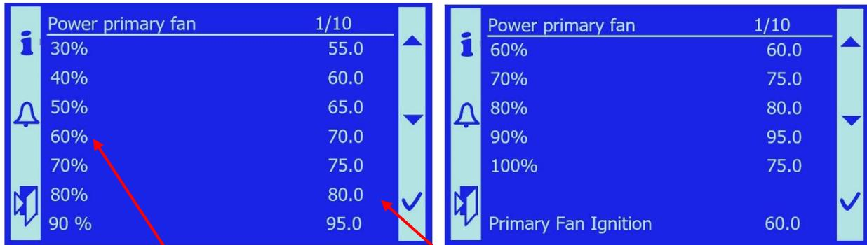
For given boiler power defined fan output is set. For primary fan and the secondary fan also the desired output during ignition is set.
