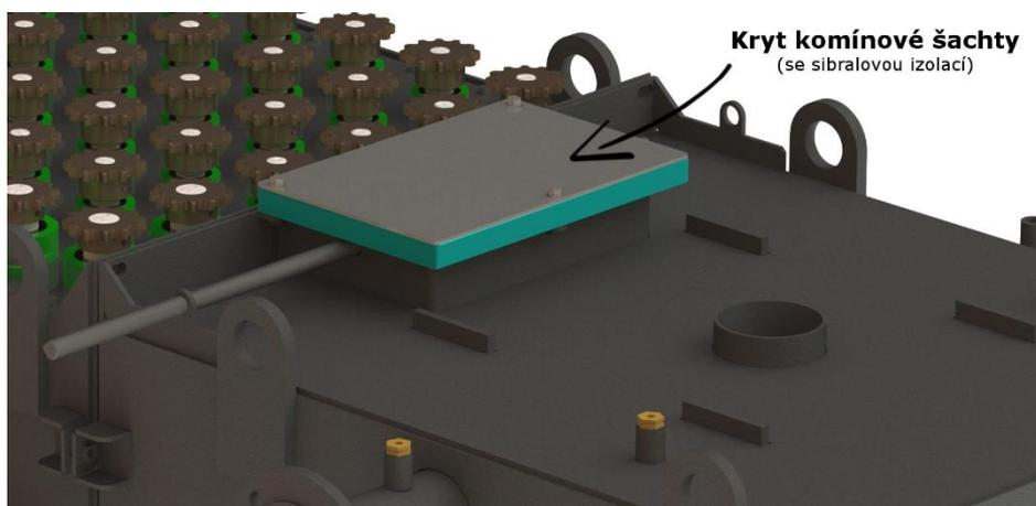
4. Insert the internal inspection door.
