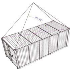
Figure 1 – Lifting angle for top ISO corners
