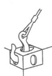
Figure 2 – Lifting by top ISO corners
