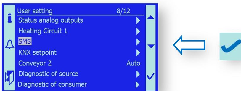
After the modem is connected and service activated, up to 4 phone numbers can be entered. However, SMSs will only be sent to one current phone number.
