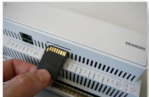
(take out the card the same way press the card against a spring strain, and the card will pop out from SD slot).
