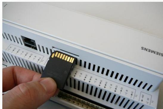
(take out the card the same way press the card against a spring strain, and the card will pop out from SD slot).
