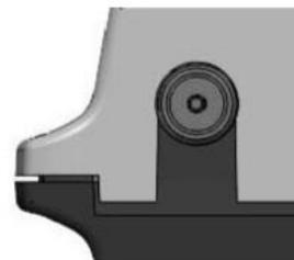
Figure 10: Antenna connector
