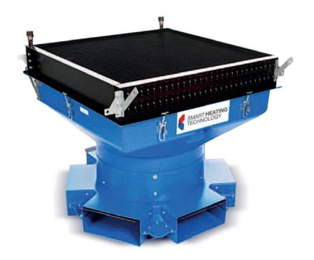
The Smart Air Heaters 360° unit consists of high efficiency heat exchanger, axial fan and a unique designed distribution device. Hot water is supplied from an external boiler and passes the heat exchanger. The fan sucks the air from inside the building through the heat exchanger and pushes the warm air equally through the 6 air outlets.
