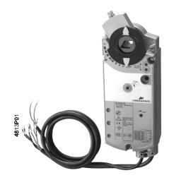
Electromotive rotary actuators for two-position control, nominal torque 16 Nm, spring return to fail-safe position, operating voltage AC 24 V or AC 230 V, for two-position control, span mechanically adjustable between 0...90°, pre-wired with 0.9 m long connection cables.
