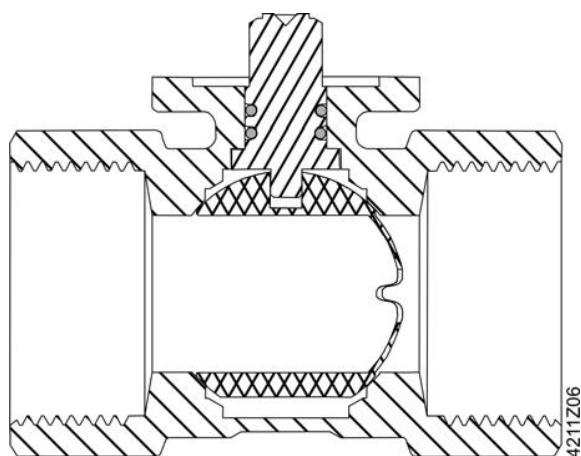
Ball with integrated control characteristic
