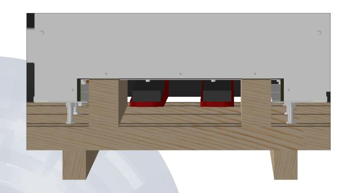
8. Direct your forklift's forks under the Combustion Chamber/Exchanger section – between the supporting wooden beams!
