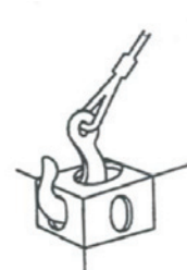
Figure 2 – Lifting by top ISO corners
