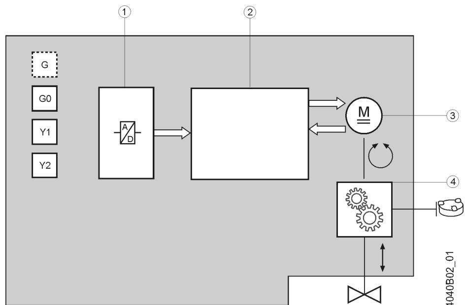
A 3-position signal drives the actuator via connection terminals Y1 or Y2. The required position is transferred to the valve.
