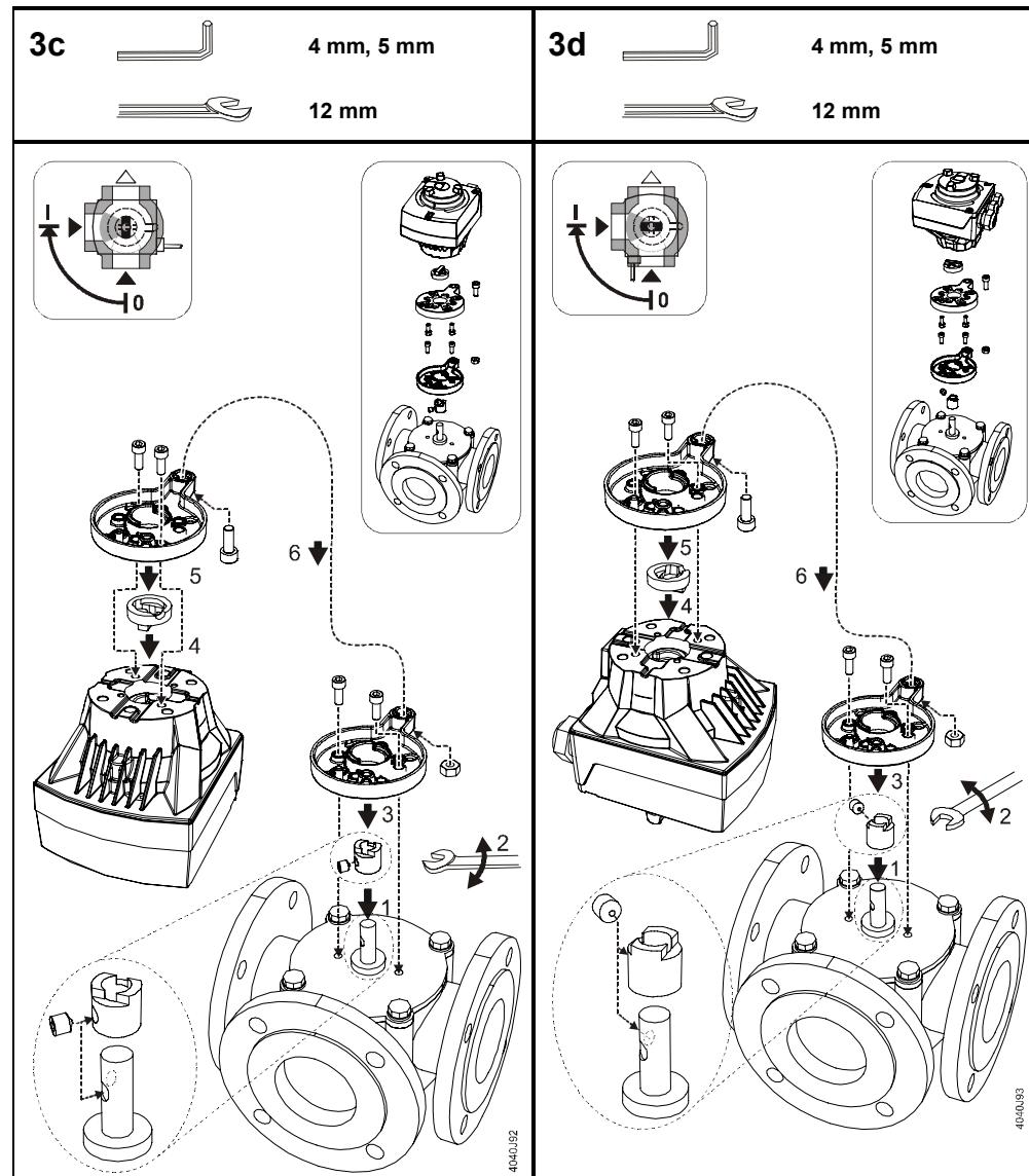
For further mounting positions of VBF 21.. and routing of the connection cables the rotary actuators and adapters must be mounted according to the sketches above.
