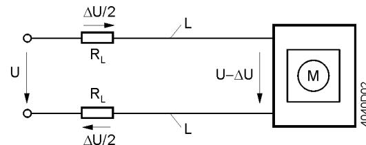
The following diagram can be used to determine the cable lengths and wire cross-sectional areas.
