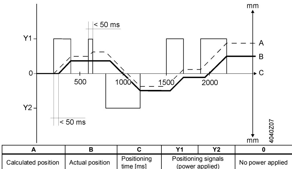
Accurate position feedback is made possible with the help of a potentiometer (page 53).
