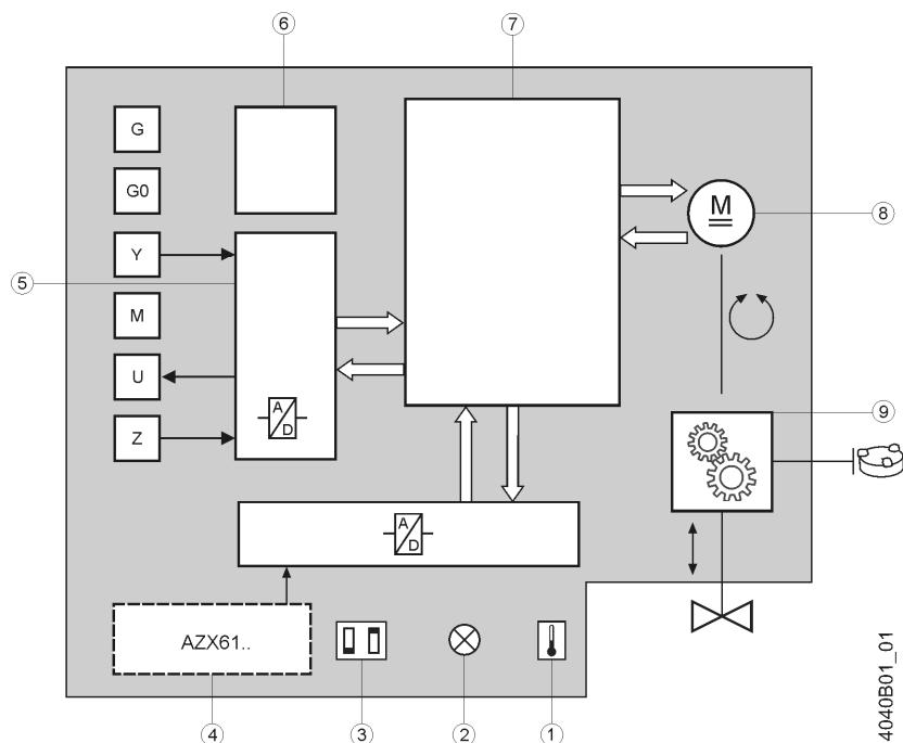
The modulating positioning signal drives the actuator steplessly. The positioning signal range (DC 0...10 V / DC 4...20 mA, 0...1000 Ω) corresponds in a linear manner to the positioning range (fully closed...fully open, or 0...100 % stroke).
