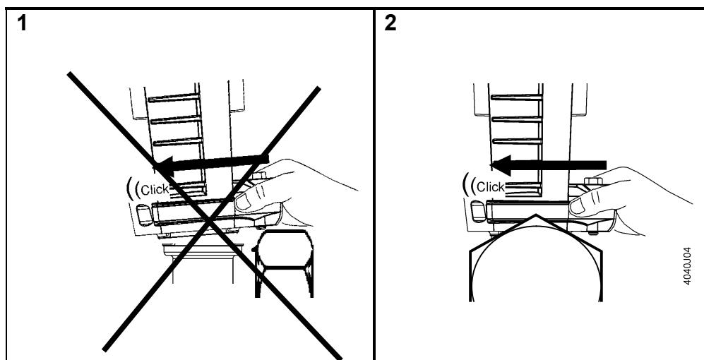
On threaded valves it's possible that the actuator is missaligned on the valve due to a collision with the fitting. If so, please take care for correct mounting, either by turning the actuator or by adjusting the fitting (e.g. use a second sealing to change fitting position).
