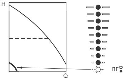
**Fig. 31** Minimum curve duty
