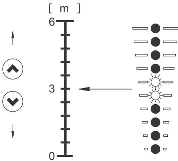
**Fig. 28** Setpoint set to 3 m, differential-pressure control
