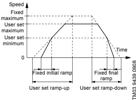
Fig. 70 Ramp-up and ramp-down
