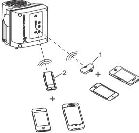
**Fig. 34** Grundfos GO communicating with the pump via radio or infrared connection, IR
