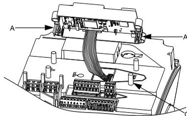
Fig. 86 Positioning the plastic cover
