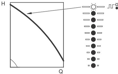
**Fig. 30** Maximum-curve duty
