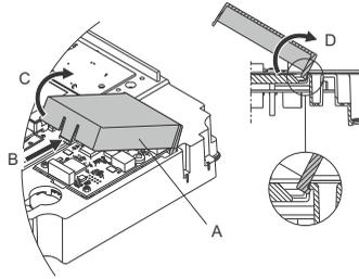
**Fig. 74** Removing the CIM cover
