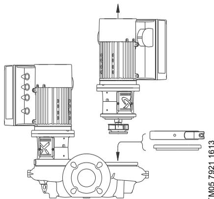
Fig. 88 Fitting the blanking flange
