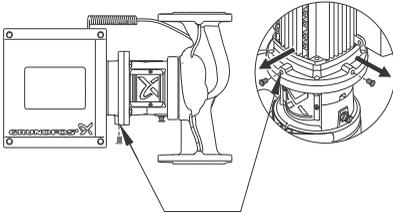
**Fig. 6** Drain hole in motor flange
