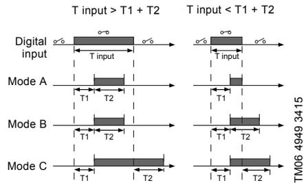
**Fig. 60** Duration timer function of digital inputs
