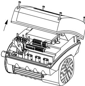
Fig. 83 Removing the terminal box cover
