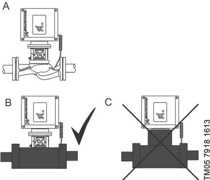
Fig. 12 Insulation of TPE2, TPE3 pumps
