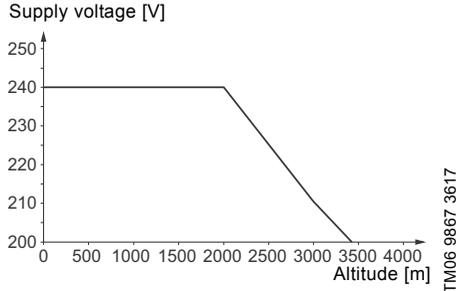
**Fig. 26** Supply voltage for single-phase motor in relation to altitude
