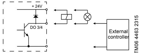
**Fig. 59** Example of configurable digital inputs or outputs
