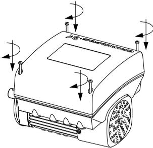
Fig. 87 Fitting the terminal box cover
