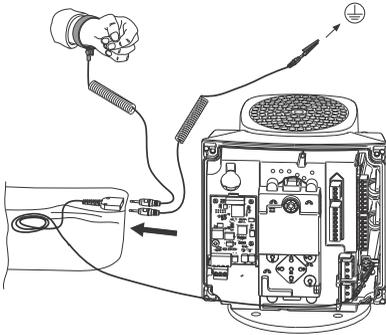
**Fig. 72** Antistatic service kit
