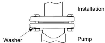
**Fig. 3** Use of washers for oval bolt holes
