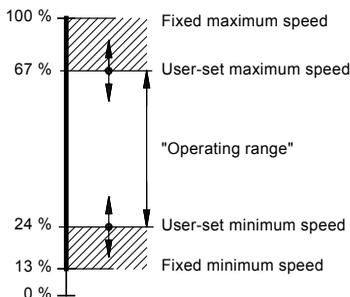
Fig. 61 Example of minimum and maximum settings
