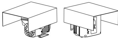
Fig. 14 Examples of covers, not supplied by Grundfos
