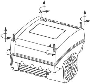
Fig. 82 Loosening the screws
