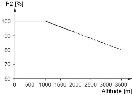
**Fig. 24** Motor output power in relation to altitude
