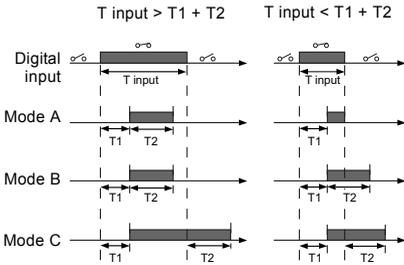
**Fig. 58** Duration timer function of digital inputs
