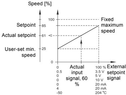
**Fig. 63** Example of setpoint influence with constant curve
