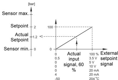
Fig. 62 Example of setpoint influence with sensor feedback
