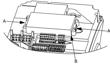
Fig. 84 Lifting the plastic cover
