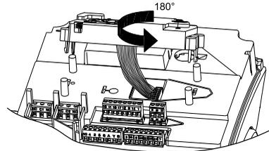
Fig. 85 Turning the plastic cover
