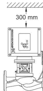
**Fig. 4** Required clearance above the motor
