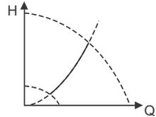
If an external controller is installed, the pump is able to change from one constant curve to another, depending on the external signal.
