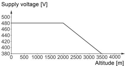
**Fig. 25** Supply voltage for three-phase motor in relation to altitude
