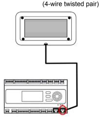
Connection for POL871.72 Cable length Cable type Cable with RJ45 plugs on both sides 1.5 m Separated Cat-5 Ethernet cable with two RJ45-plugs (8-wire twisted pair)
