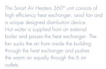
The amount of air and the directions can be adjusted by the flaps inside each air outlet. The units are hanging in the middle of the building whereby an ideal distribution is guaranteed to all corners in the building.
